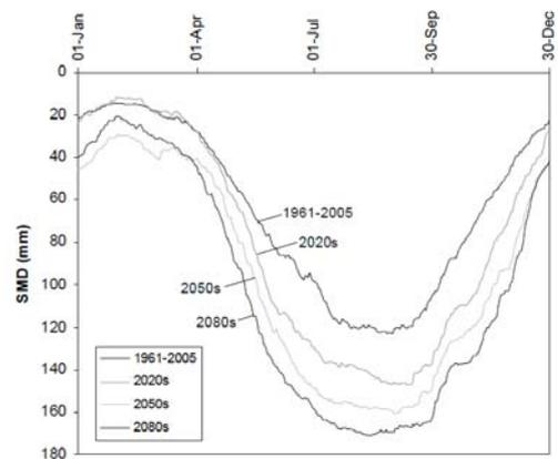
*Estimates of Soil Moisture Deficit by D. Clarke and J.A. Smethurst. (2010) "Effects of climate change on cycles of wetting and drying in engineered clay slopes", v. 43; p. 473-486 published by The Quarterly Journal of Engineering Geology and Hydrogeology*
